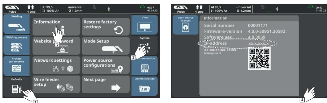
**1** Presettings / System/Information ==> note down IP address of the welding machine
